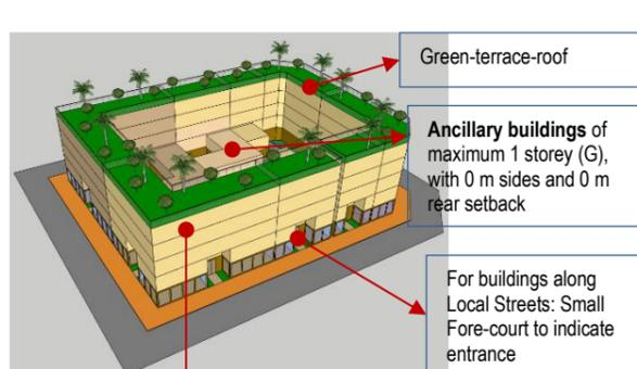
**Main buildings:** Compact low-rise buildings maximum G+4, with main buildings are built close to the edge of the block and attached to the adjacent buildings, creating a strong sense of wall and perimeter block
